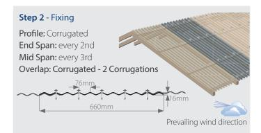
OneShot® & Clearfix, a choice in fixing, Self Drilling 50 mm Screws save up to 50% on installation time.
